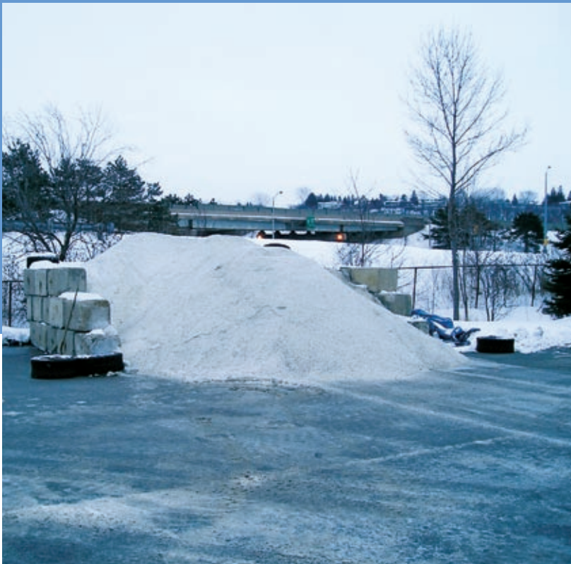
Poor, uncovered salt storage can result in significant losses and negative environmental impacts.
